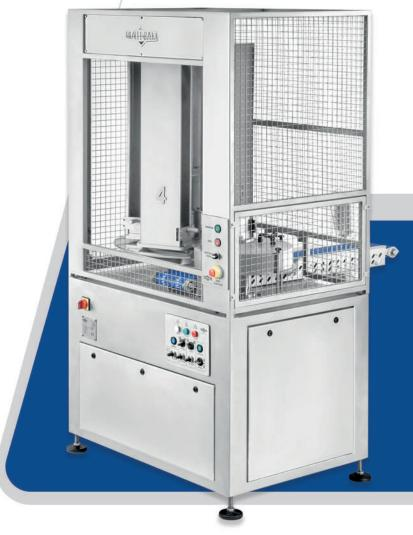
Designed for cutting boneless products. The product temperature can range from -10 to  $0^{\circ}\text{C}$  depending on the product morphology and desired thickness.
